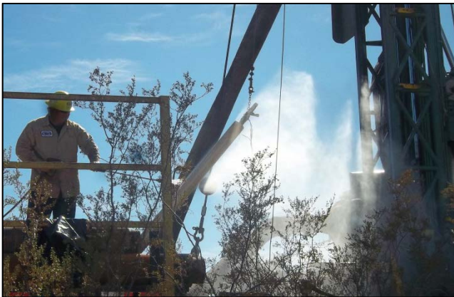
The 1.5-horsepower pump used for depth-specific sampling was decontaminated prior to each use via power washing.
