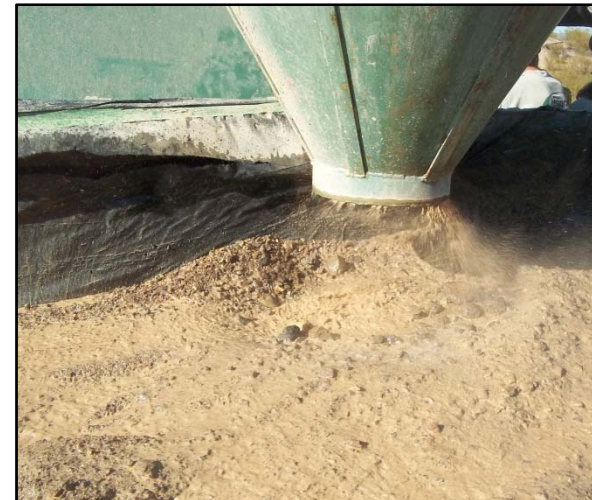
Drill cuttings and water generated from drilling enter an energy dissipating cyclone and are deposited into a water tight roll-off bin. Samples were collected at 5-foot intervals.
