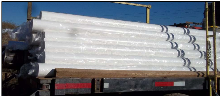
Factory sealed, 5-inch, Schedule 80 PVC well casing and well screen with 0.040-inch horizontal slots.
