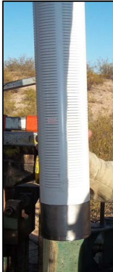
Factory sealed, 5-inch, Schedule 80 PVC well casing and well screen with 0.040-inch horizontal slots.
