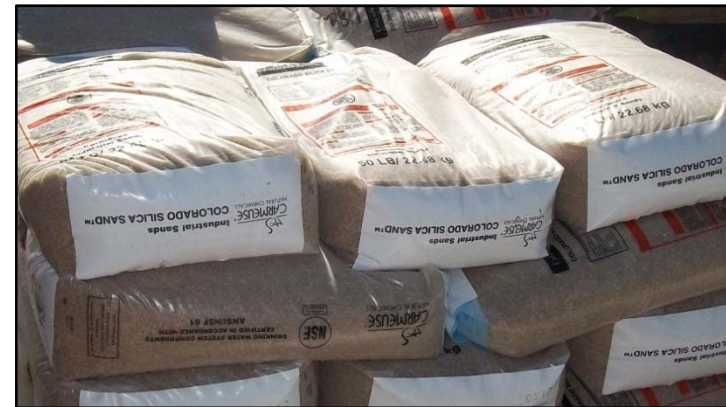
Annular materials included hydrated bentonite pellets, 8-12 mesh sand, #60 (fine) sand, bentonite grout and cement grout, which were gravity fed between the drill pipe and the well casing.
